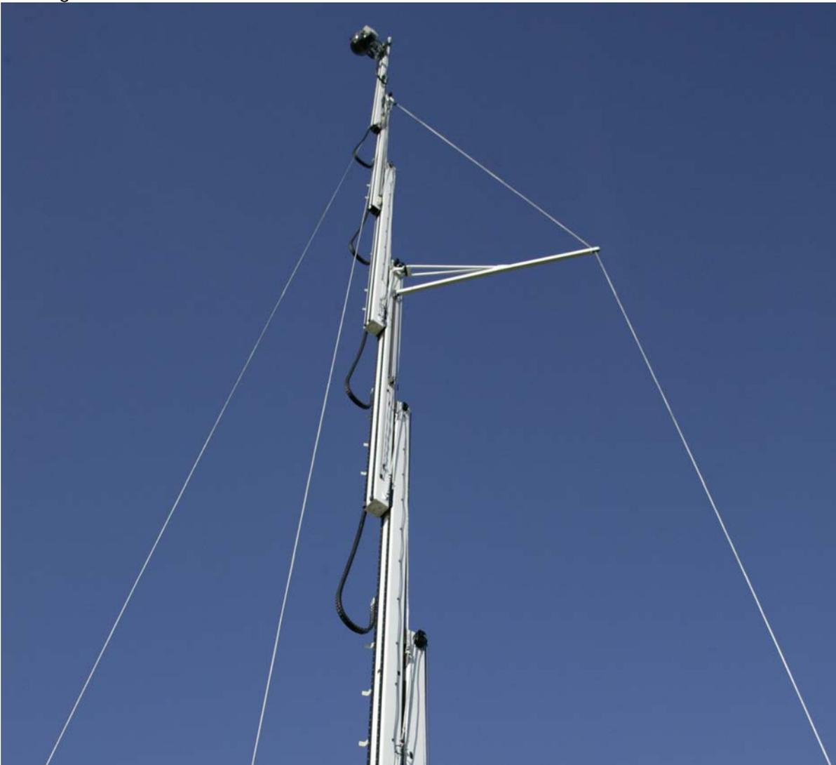
Stabilisation control is taken care of with four Kevlar guy ropes that are fixed at the top of the mast near the camera platform and are controlled from servomotor driven geared
