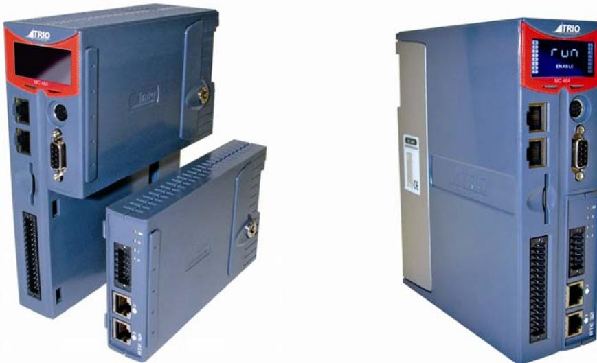
As the latest and most advanced addition to Trio's *Motion Coordinator* family, the new MC464 is a multi-axis motion and machine controller featuring a high performance 64-bit processor in a modular design that provides OEMs and automation system integrators with a flexible choice of servo and stepper drive interfacing combined with a wide selection of Fieldbus protocols - plus programming flexibility that includes Trio's own Trio BASIC or industry standard IEC 61131 runtime.
