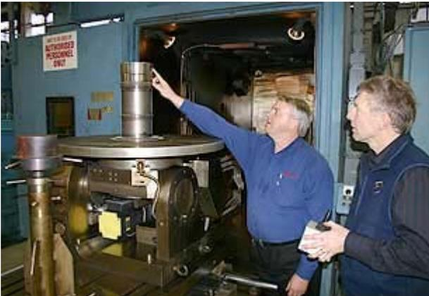
There is a beam on a number of very happy faces across at Air New Zealand Gas Turbines facility at Auckland International Airport these days that has nothing to do with the glow emitted from the 'cathode ray tubes' atop the recently upgraded 30-year old, 200,000 volt, Sundstrand welding machine, which is still one of the biggest in the world.
